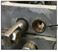
High/Low gear shift rod removed. Be VERY careful to avoid dropping any parts or debris into the transmission.
