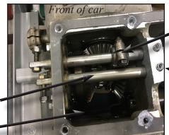
Front, shorter shifting rod that controls forward or reverse gear selection. You will need to loosen this nut and bolt to remove the forward/reverse shift rod.
