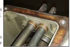
Since there is no pressure in the case, install the lip of the seal face out, it will act as a wiper/scraper to keep dirt out. Put a little lube on the seals (Inner Di-
