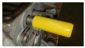
Using the bushing driver/spacer tool (yellow), slide the end with the 1/8" step over one of the shift rods. Using a small hammer drive, the bushing into the case until the shoulder of the tool hits the case. This doesn't require much force so take it easy. The bushing will be inset about 1/8" on each shift rod, creating a space for the seal. If you are using a socket or other device, drive the bronze bushing only 1/8" inside the case.
