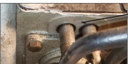
Both seals have been installed and fully seated within the wall of the transmission case. All that's left now is to reinstall the shift levers and the work is finished
