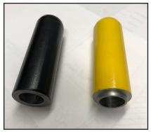
On the black Seal Installer, the wide, flat surface fully contacts the seal so there is nearly equal pressure on it as it is driven into the bushing space. This face will also contact the case and prevent you from over driving the bushing inside the case.
